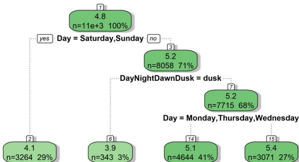
Figure 7. Decision tree for speed difference using temporal variables when only considering those 15-min periods when conditions are LOS A, B, or C.
