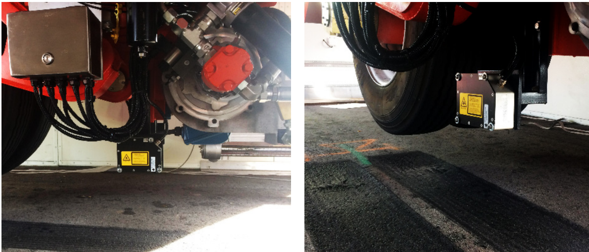
Figure A-3. Laser profiler mounted on HVS carriage.
