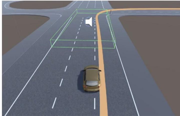
Figure 7. Geofence to indicate audio and visual cues of pedestrian crossing. Participants could not see the geofenced areas on their HMI version.
