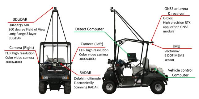
Figure 16. Golf car retrofitting architecture for slow speed tests.
