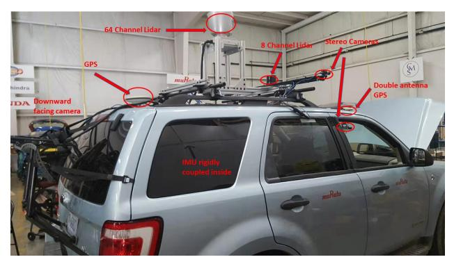
Figure 15. Equipment installation picture of the test vehicle.
