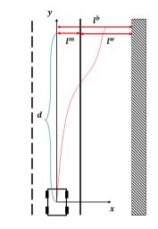
Figure 2. Roadside space estimation illustration.
