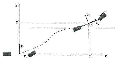
Figure 9. Model for EKF estimation.
