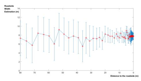
Figure 6. The estimated mean roadside width and its  $3\sigma$  errors as the vehicle slows down.
