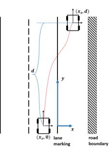
Figure 7. Illustration of emergency stop navigation control problem
