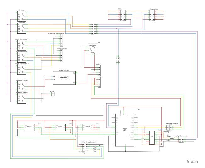
Figure 17. Drive-by-wire controller wiring configuration.
