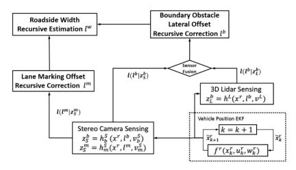
Figure 3. Roadside perception system configuration.
