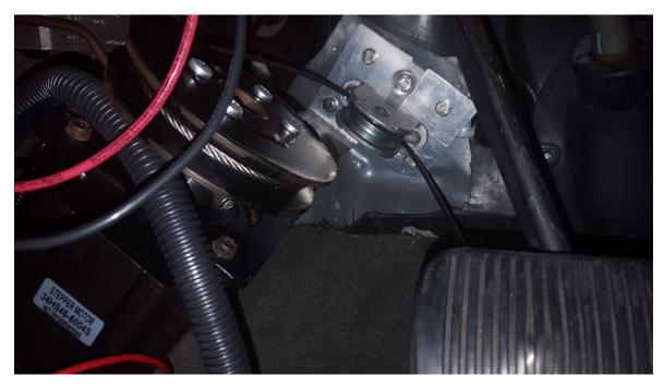
Figure 18. A pulley is drilled and mounted on the steel hub of the motor shaft for brake actuation.
