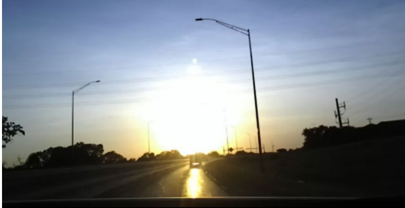
Figure 1: Glare from sun severely affecting visibility as seen from an RGB camera while driving.
