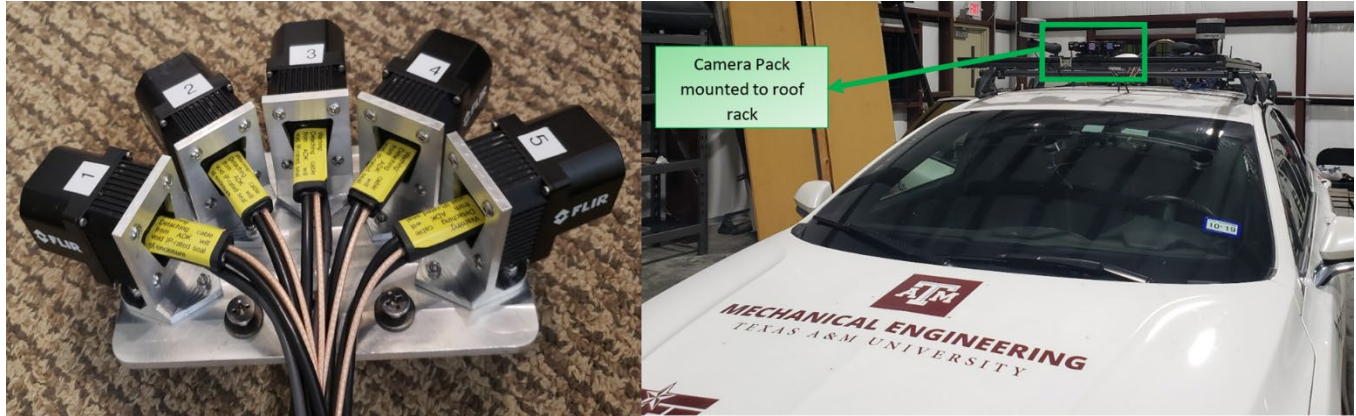
Figure 4: Machined product and mounting location.
