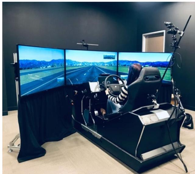
**Figure 1. The driving simulation lab setup including the driver’s seat and forward view screens. Note that the eye-tracking system is positioned on top of the dashboard.**
