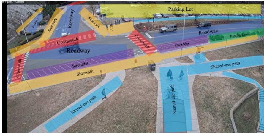
Figure 10. Photo with color labels. Color-coded infrastructure elements at camera location Ambler Johnston Hall East-Wing.
