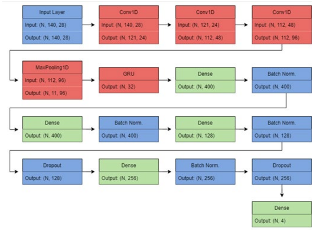
Figure 6. Diagram. Neural network diagram – glance only model.
