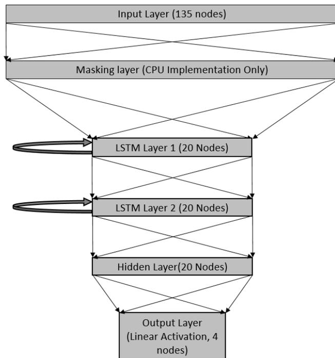
**Figure 9. Diagram. Final model architecture.**
