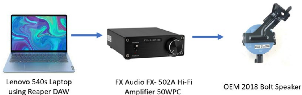
Figure 4. Factory modified system diagram.
