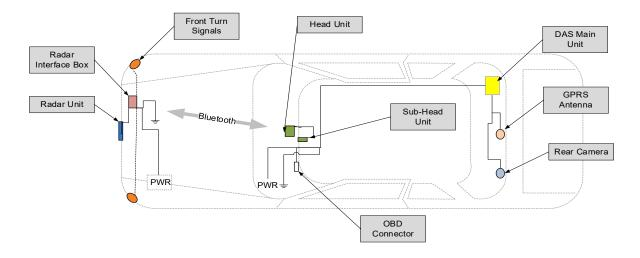
Figure 2. DAS component locations in the vehicle.
