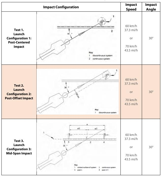
Table 11. EN 1317-8 Technical Specification Test Impact Configurations
