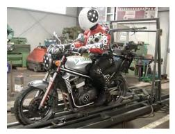
Figure 30. Test sled in upright position with motorcycle and dummy (Peldschus et al., 2007).
