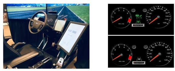
Figure 6. Photos. Left: Driving simulation lab setup including the quarter-cab, automation control screen (on the right side of the figure), and the eye-tracking apparatus (mounted above the instrument console near the steering wheel). Right: Instrument cluster when the automation is on (top figure) and is off (bottom figure).
