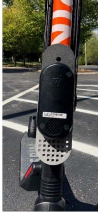
Figure 1. Photo. MicroDAS installed on a Spin scooter.
