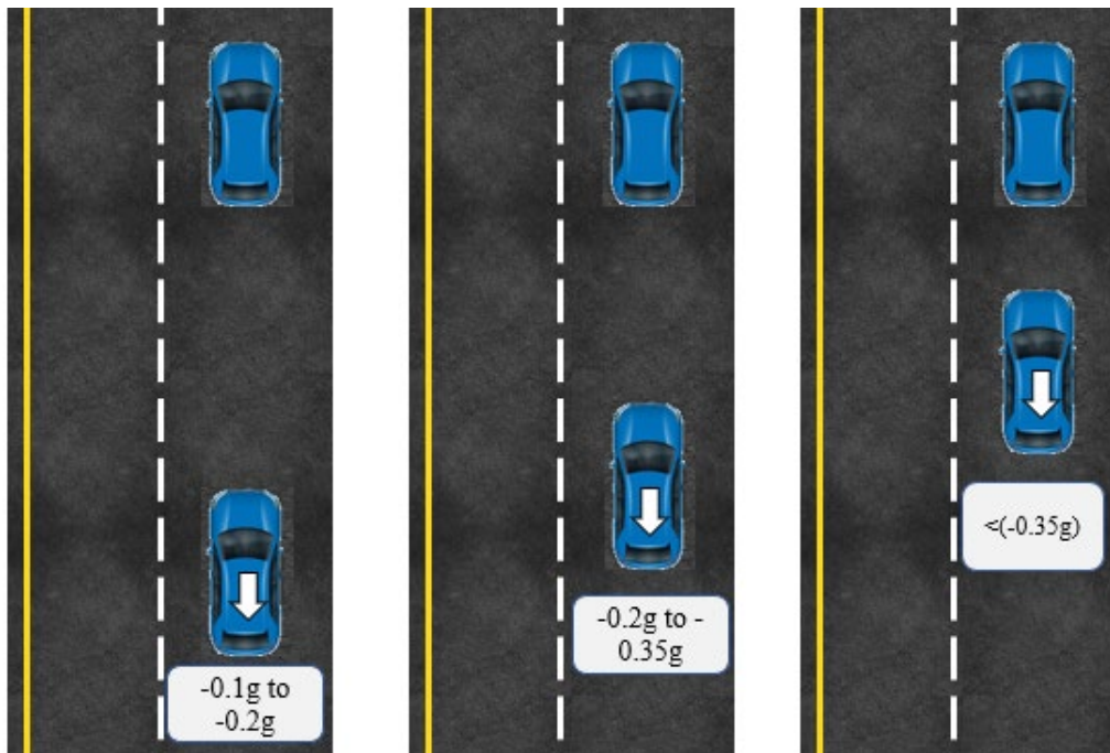
Figure 2. Schematic defining the concept of longitudinal deceleration.
