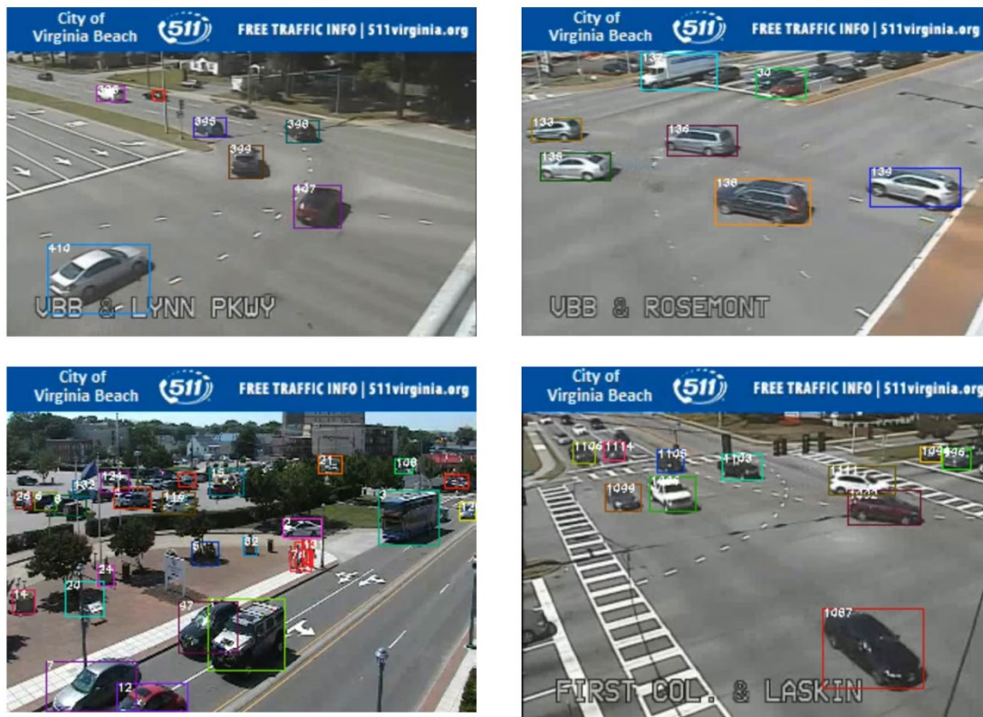
Figure 8. Example of object tracking from DeepSort.
