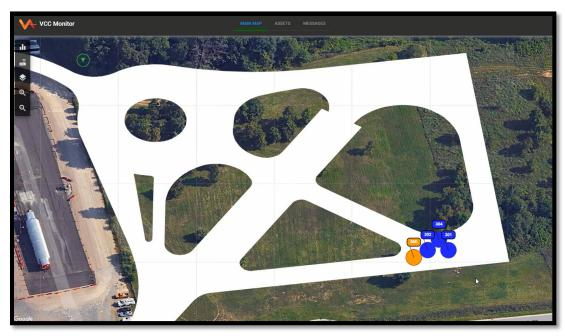
Figure 3. A picture of VCC Monitor, VTTI's web-based situational awareness tool that displays the real-time locations of UWB anchors and mobile tags (blue circles) and CAVs (orange circle).
