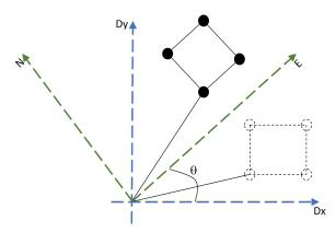
Figure 2. Graphical representation of the rotation process utilized to convert from X/Y plane from the DecaWave sensor into the WGS84 GPS north/east plane.
