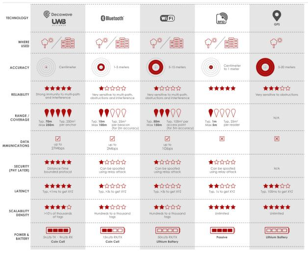
Figure 12: Decawave UWB specs (https://www.decawave.com/technology1/)
