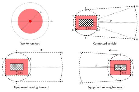
Figure 7. Representation of the safety areas designed for each WZ actor.
