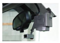
Figure A2. Radar and camera units used in the SHRP 2 Naturalistic Driving Study.
