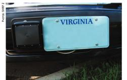
(Left:) A forward radar unit. mounted near the license plate, is among the datagathering devices installed in participant vehicles.
