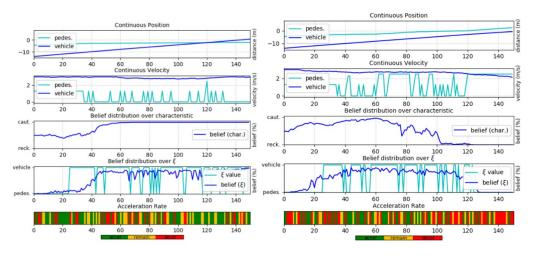
(a) (b)Figure 4. Graphs. Simulation results showing (a) vehicle executing a policy, interacting with a cautious pedestrian, and (b) vehicle executing a policy, interacting with a reckless pedestrian.
