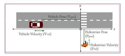
Figure 3. Diagram. Bird's eye view of crossing scenario.
