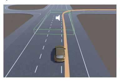
Figure 7. Geofence to indicate audio and visual cues of pedestrian crossing. Participants could not see the geofenced areas on their HMI version.
