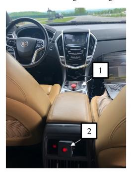
Figure 4. Stop button locations in the test vehicle.
