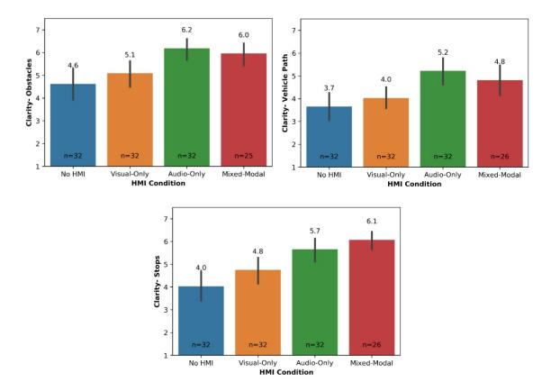
Figure 11. HMI condition compared to how clear it was at communicating the presence of obstacles in the roadway (top-left), the planned vehicle path (top-right), and intention to stop (bottom).
