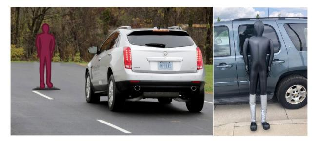
Figure 8. HV-REMO base on the Smart Roads (left). Soft target attachment used for this project (right).
