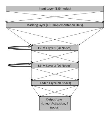
Figure 9. Diagram. Final model architecture.
