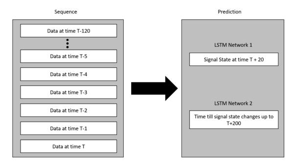
Figure 7. Diagram. Sequences and prediction variables.
