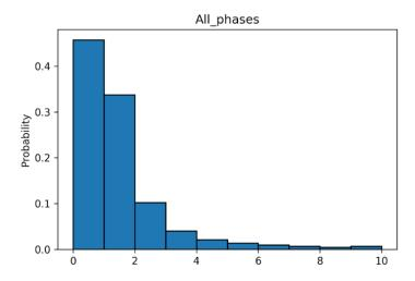
Figure 21. Histogram. Error distribution in seconds for mean absolute error function for 39-day data.
