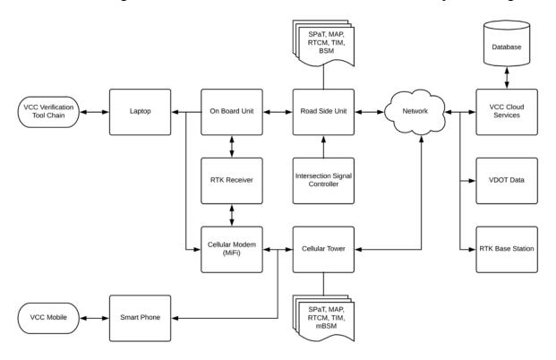
Figure 2. System diagram.
