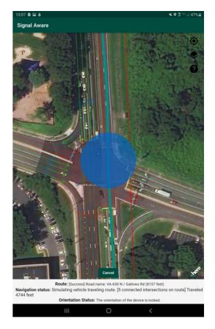
Figure 23. Screenshot. Prototype mobile application GUI - SPaT and MAP.
