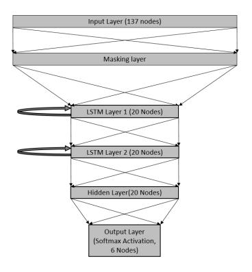
Figure 8. Diagram. Preliminary prediction model architecture.
