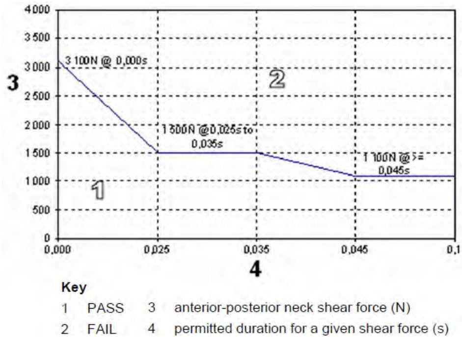
Figure 33. EN 1317-8 Technical Specification Force and Moment Criteria
