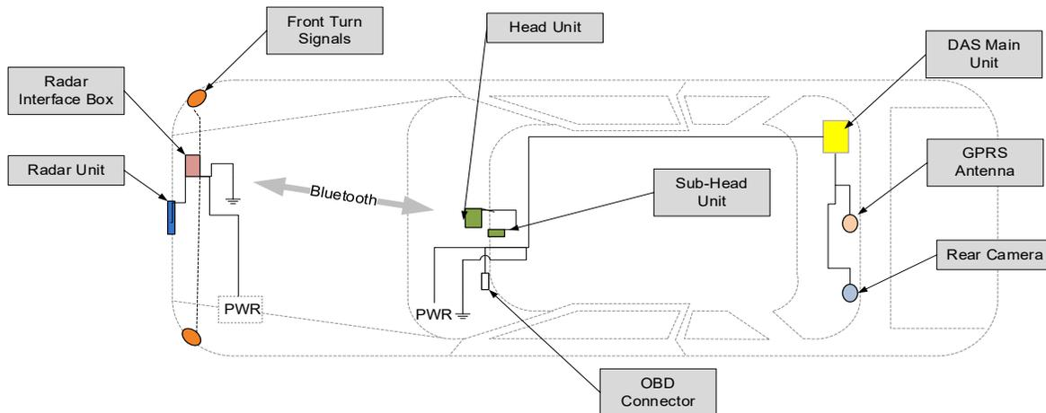
**Figure 2. DAS component locations in the vehicle.**
