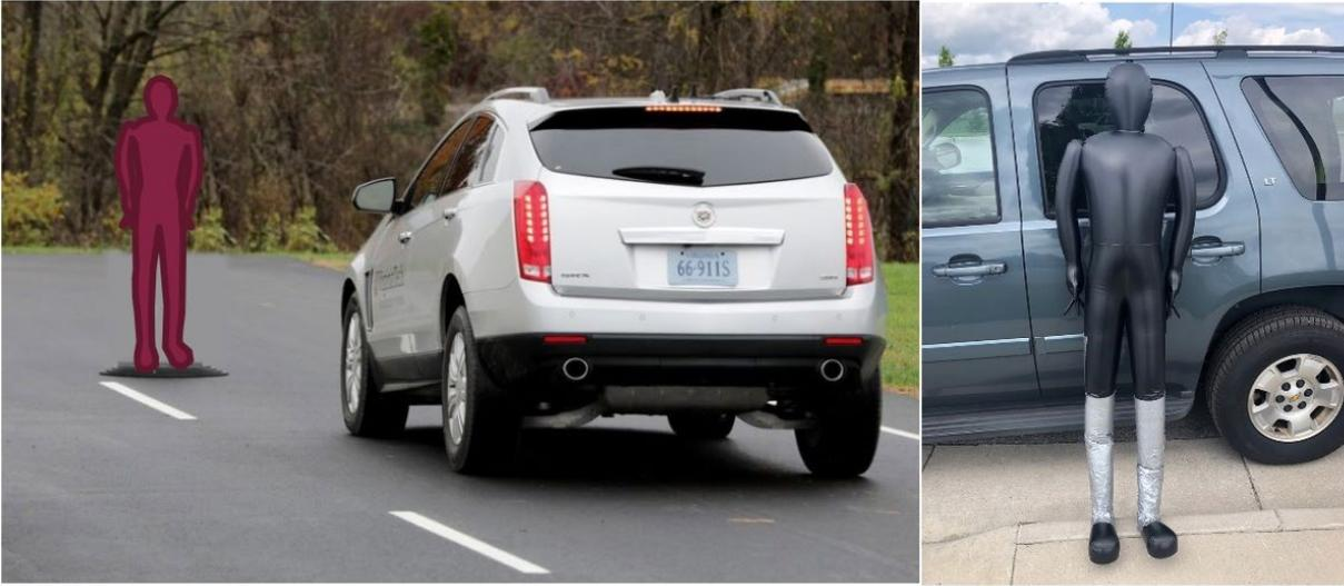
Figure 8. HV-REMO base on the Smart Roads (left). Soft target attachment used for this project (right).
