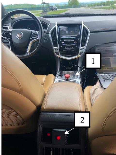
Figure 4. Stop button locations in the test vehicle.
