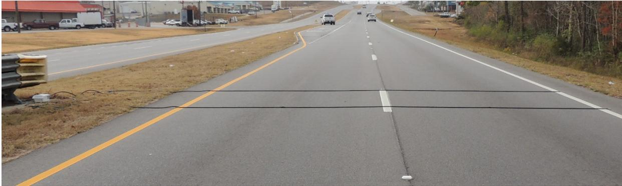
**Figure A1. Example of road tubes installation.**
