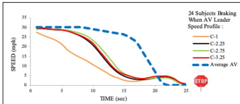
Figure 8. Participants average braking speeds vs AV leader speed profiles.
