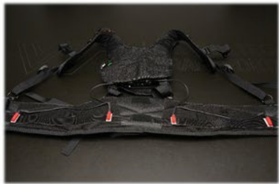
Smart Vest tactors attached to the belt using a Velcro strip allowing adjustments, if needed
