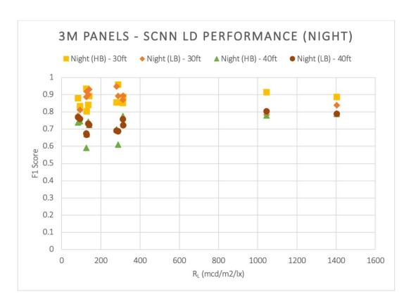
Figure 25: Plot of LD performance vs retroreflectivity (R<sub>L</sub>) for the 3M pavement panels.
