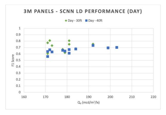
Figure 24: Plot of LD performance vs diffused reflectance (Q<sub>d</sub>) for the 3M pavement panels.
