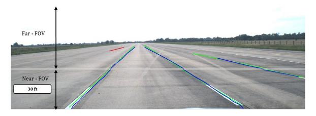
Figure 9: Image showing the area-split for near FOV vs far FOV evaluations.
