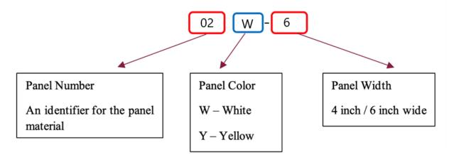
Figure 3. Panel identification scheme.
