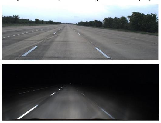
Figure 5: Images of 40 ft gap pavement markings on 35L (Set 2: 06W-6 on left and 02W-6 on right) during day (above) and night (below).
