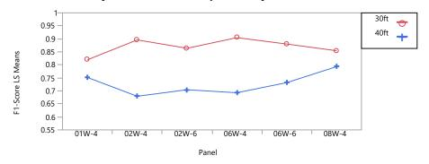
Figure 12: Plot of least square mean F1-score capturing the effect of two-way interaction of panel spacing on panel material for nighttime LD performance.
