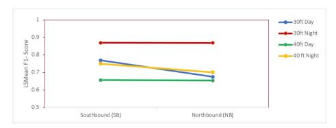
Figure 15: Plot of least square mean F1-score capturing the effect of 2-way interaction of panel spacing and driving direction on LD performance.
