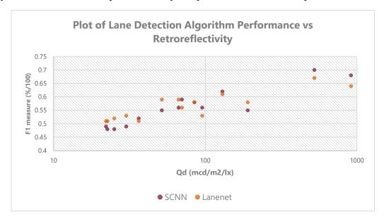
Figure 23: Plot of lane detection performance of SCNN & LaneNet algorithms (measured as F1 score) vs continuous  $R_{\rm L}$  data for pavement markings on RELLIS 35L.
