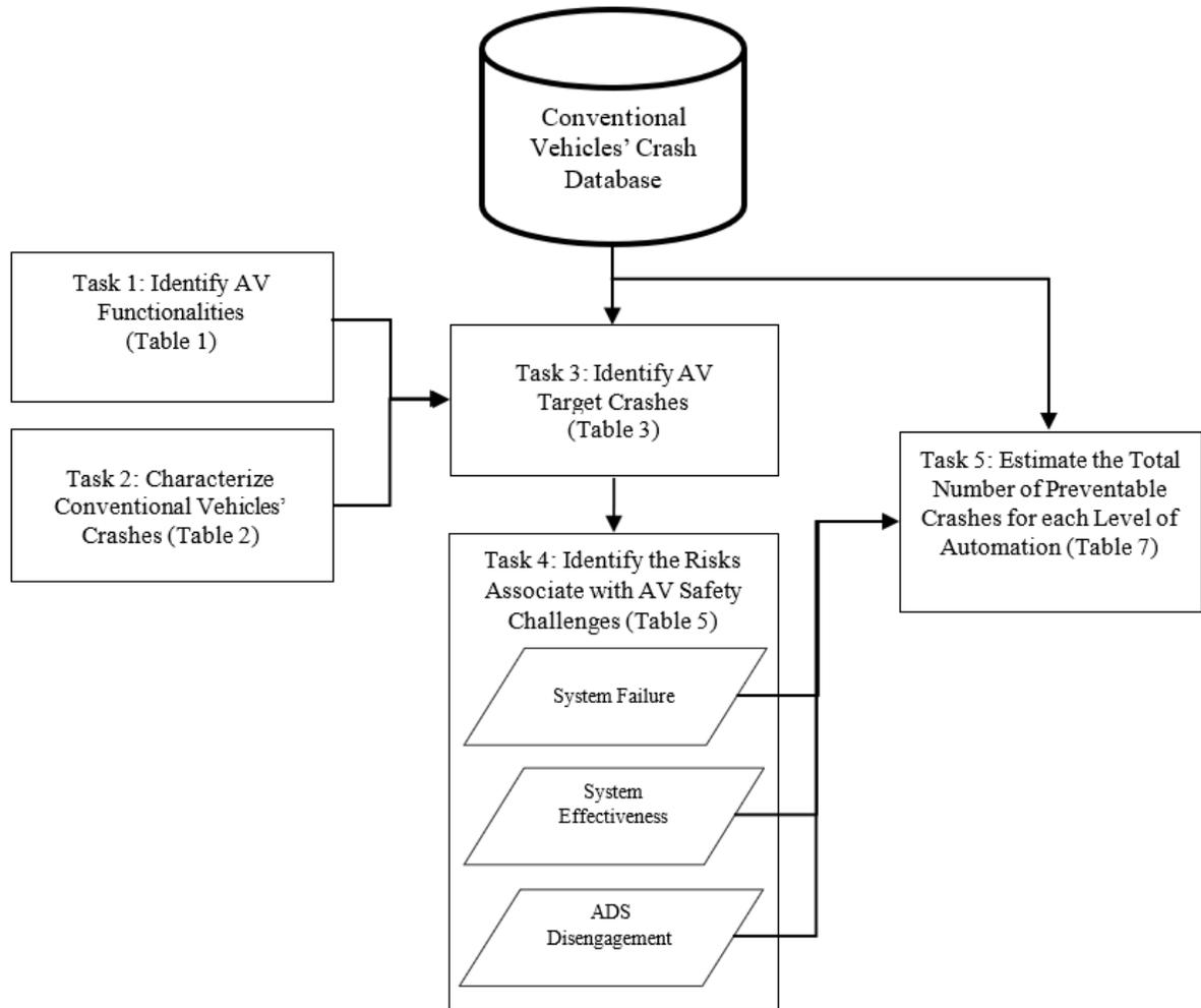
Figure 1. Flowchart. AV safety quantification framework.
