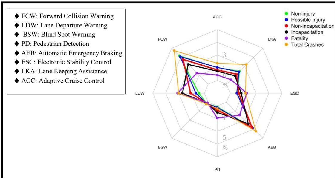
**Figure 4. Chart. ADAS estimated preventable crashes by severity.**
