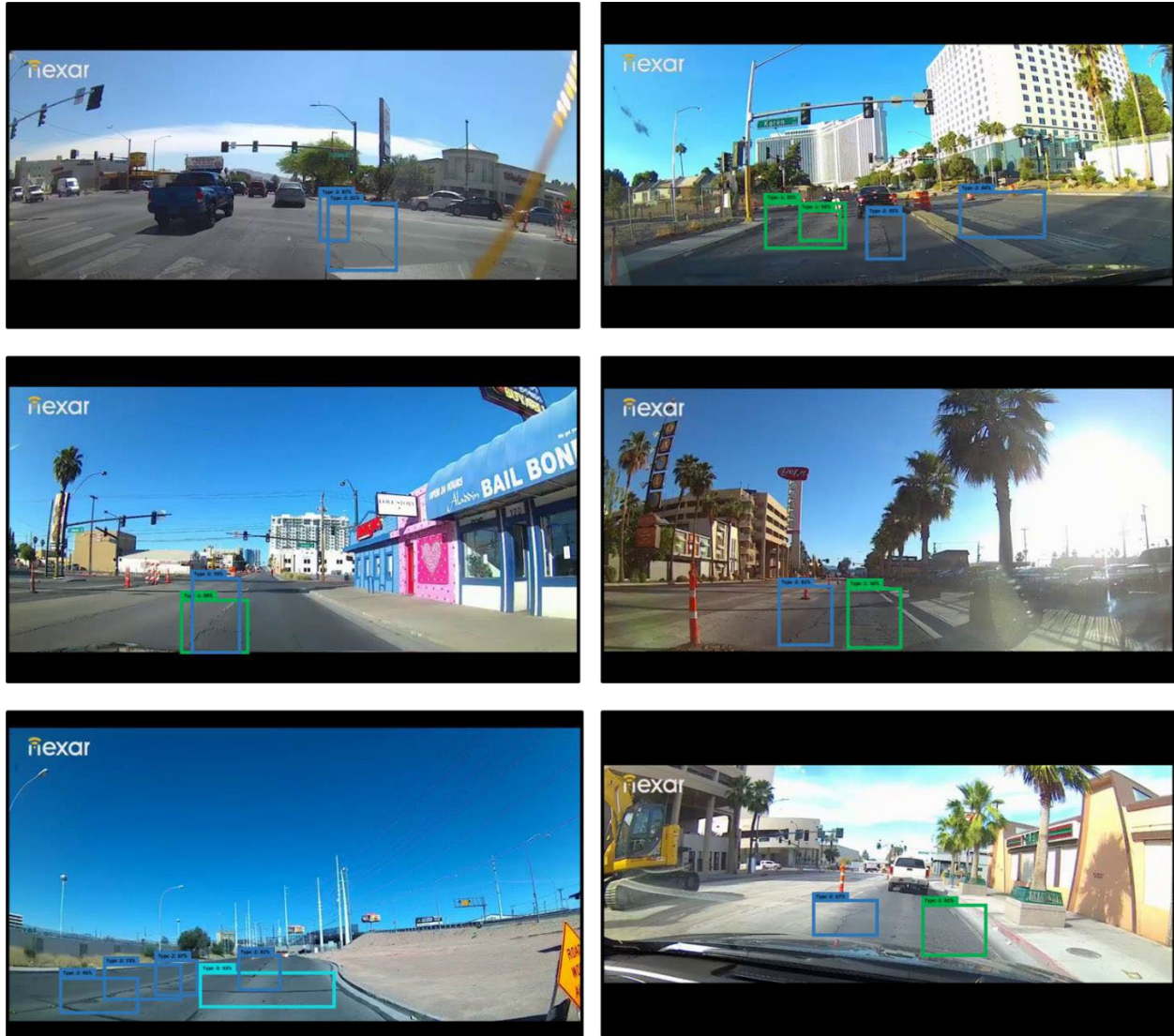
Figure 5. Examples of pavement damage detection in Nexar images.
