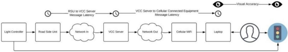
Figure 17. Diagram. End-to-end SPaT latency points.
