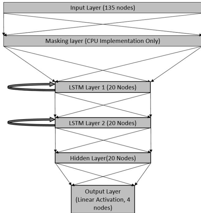
**Figure 9. Diagram. Final model architecture.**
