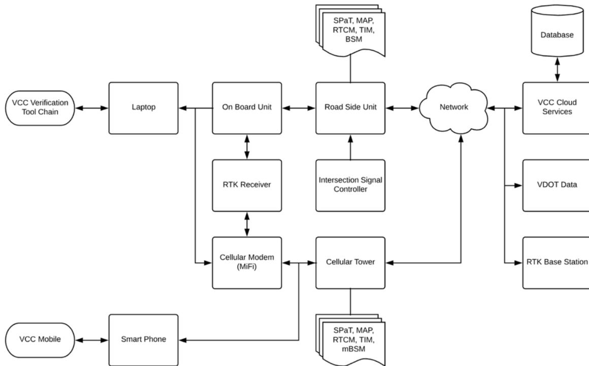
Figure 2. System diagram.
