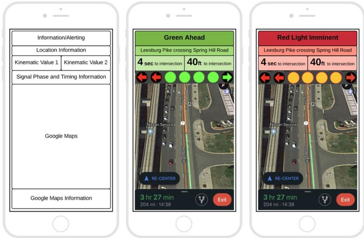
**Figure 13. Image. Conceptualized mobile application GUI.**
